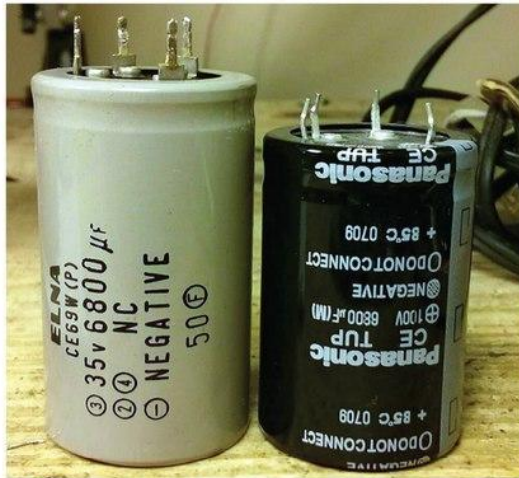
Components have come a long way in the last few decades! Left, the original snap-in capacitor; right, a drop-in replacement rated at three times the working voltage while still taking slightly less space.
